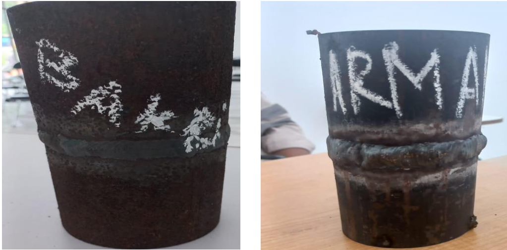
Gambar 3. Hasil Pengelasan Pipe to Pipe
